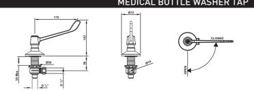
Description: Elbow action, 1/4 turn side valve with a red indice. 1/2" BSP male
