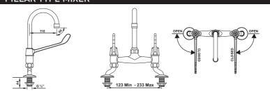
Elbow action pillar type % turn mixer with an aerated swan neck swivel outlet. %" BSP male inlets. SANS 226 TYPE 2 515-21 Description:
