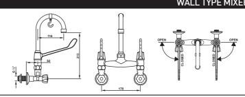
Description: Elbow action wall type mixer with angle regulating valves and a hook
