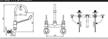
Elbow action 1/4 turn wall type mixer with a swivel outlet and a Description:
