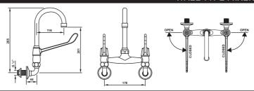
Description: Elbow action ¼ turn wall type mixer with a swivel outlet.½"
